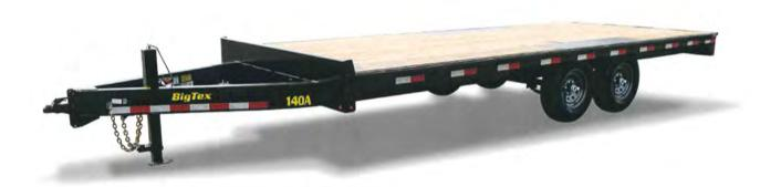
AXLE JACK (2) 7,000# Quick Lubricating w/Electric Brakes 12,000# Drop Leg Jack (Bolted On) G.V.W.R. TOP RAIL 14,000# NONE
