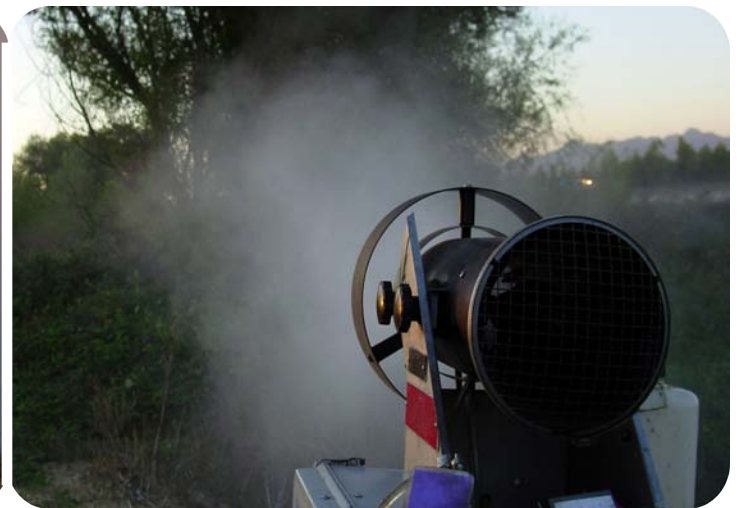
Truck mounted fogger in the wetlands west of Gridley.
